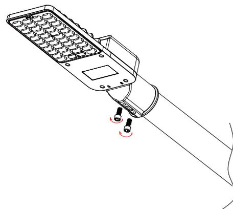
2. Loosen the the screws for fixture mounting. Stick the pole arm into the mounting tube. Fasten up the two screws evenly in a way of multiple interchange instead of one-by-one, making sure of the compliance of torque force. Installation finished.
