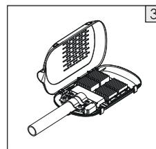
3. Loosen the four screws on the arched clamps to let pole arm stick in, then fixate it by tightening up the screws.
