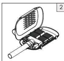
2. Undo the two M4x10 screws on the ends of the failed module.
