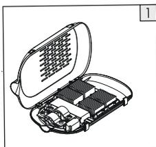
1. Undo the two buckles to open the cover.
