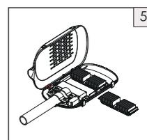
5. Tighten up the cable connector and the screws.
